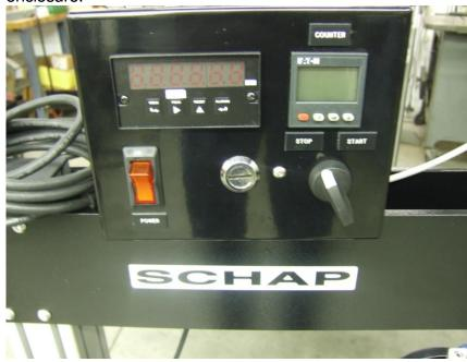
Turn on Air and set to **20 to 60 psi**. (You may need to adjust the air pressure slightly to achieve proper operation of the unit 60 psi is our recommended
