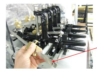
Tension Scale bar and screw. Remove these, and save in a box.
