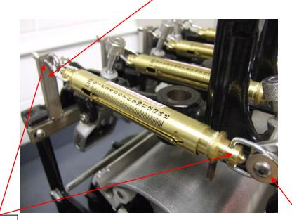
Install the scale as shown, and close the eye hook with pliers.
