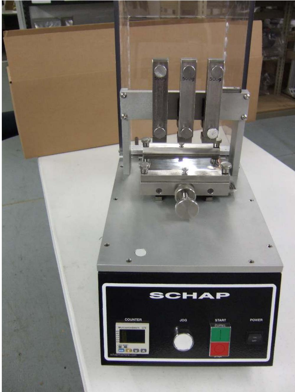
The tester is made with stainless and aluminum components so that the operator can apply moisture with the samples or during the test without causing damage to the tester.
