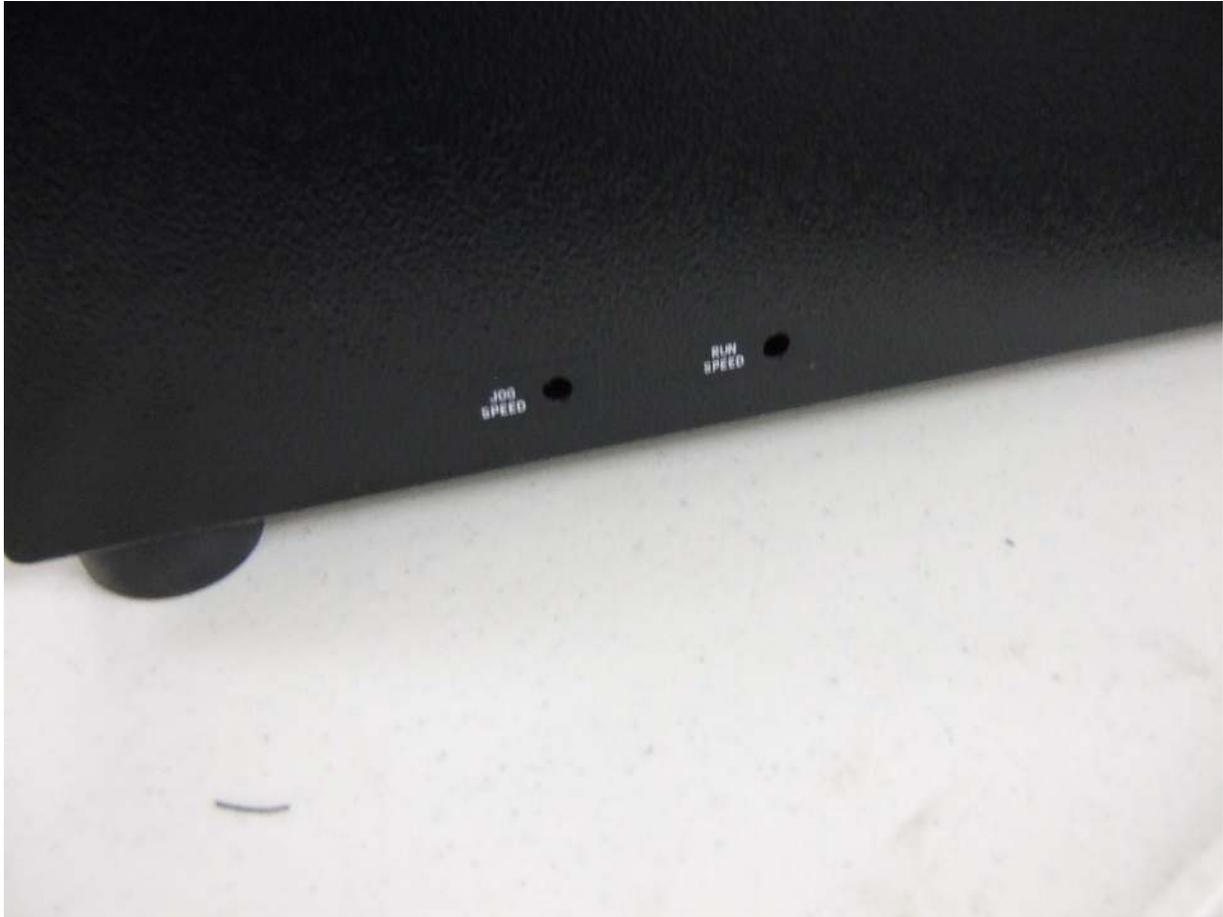
ON THE SIDE OF THE TESTER ARE TWO PLACES FOR SPEED ADJUSTMENT.
